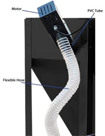
Electrically powered auger that transports fuel to the burner depending on the operating mode of the burner. The screw consists of a compact geared motor with a built-in protection against overheating tube which transports fuel until it reaches the hole through which is supplied to the flexible tube. The flexible tube is made of special heat-resistant material (which in the case of combustion does not emit toxic substances) and connects the auger and pellet burner.
